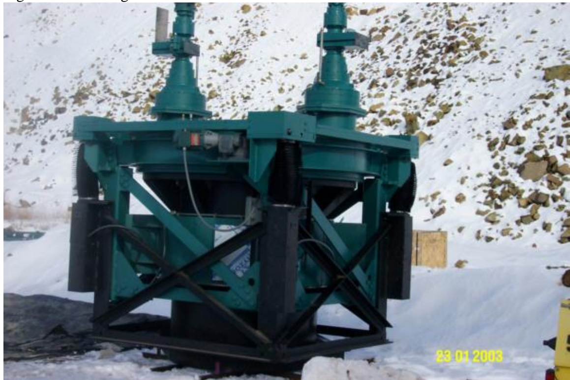
Figure 7. First Stage Clarifier Drive Mechanism
