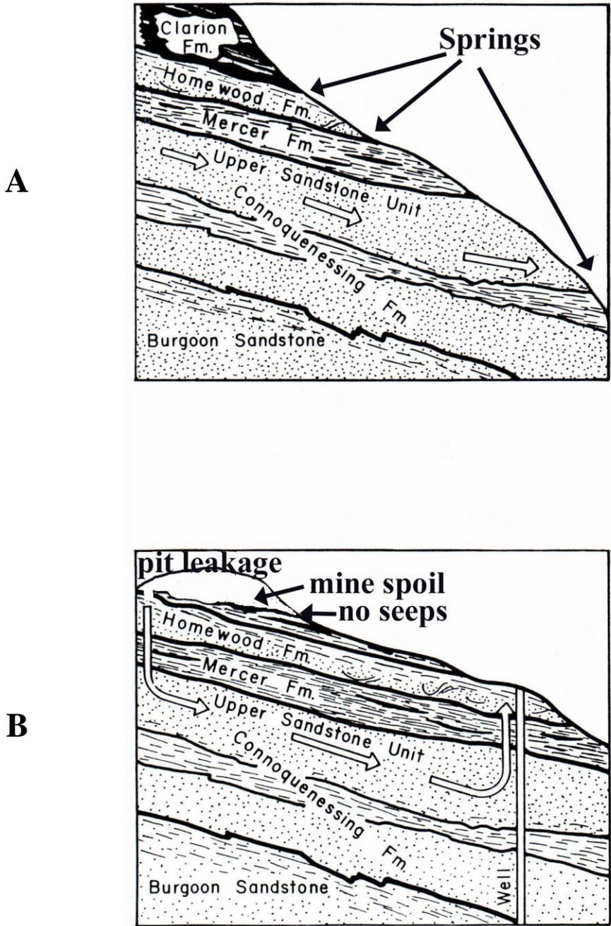
Figure 3. Typical cross section of the pre and post-mining water drainage. 3A illustrates drainage through undisturbed rock (pre-mining). 3B shows
