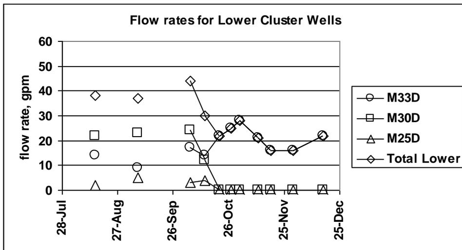
Figure 7b. Flow rates for the lower cluster of wells. The first column of symbols represents 2002 averages. The second column is pre-plugging measurements made in September 2003. Symbols connected with lines are flow rates measured during plugging activities.
