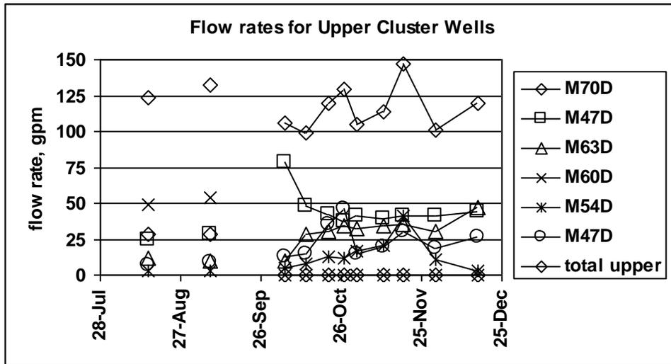
Figure 7a. Flow rates for the upper cluster of wells. The first column of symbols represents 2002 averages. The second column is pre-plugging measurements made in September 2003. Symbols connected with lines are flow rates measured during plugging activities.
