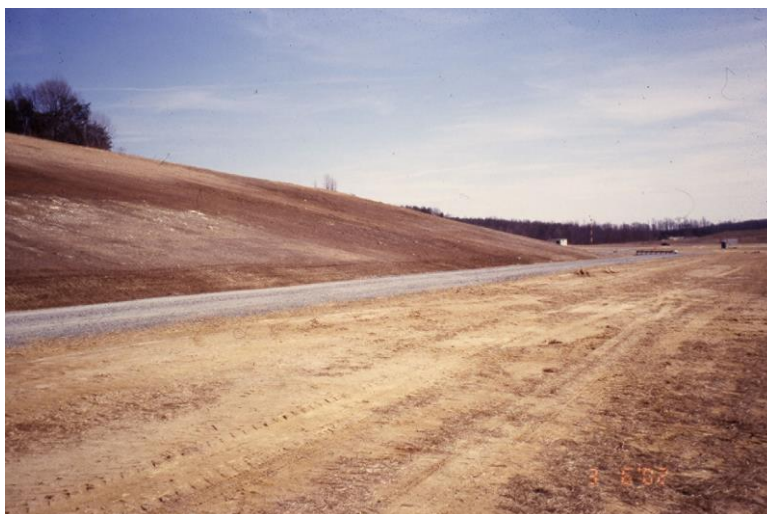
Figure 2. Barren fields resulting from the development of acid sulfate soils over disturbed sulfide-bearing Tertiary marine sediments at Stafford Regional Airport.
