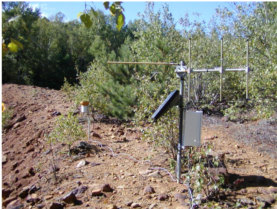
Figure 8. The instrumentation at the South Cut site, Elizabeth Mine, South Strafford, VT. This site contains a data logger, radio receiver for receiving data from other loggers at the site, and cellular transmitter for uploading all data to a database and web site at CRREL.
