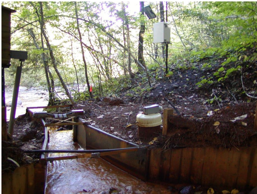
Figure 6. Measuring flow at an artesian air vent, Elizabeth Mine, South Strafford, VT. Flow emerges into a moat, then decants through a pipe into a Parshall flume.
