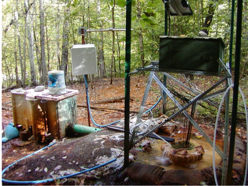
Figure 6. Measuring flow at an artesian air vent, Elizabeth Mine, South Strafford, VT. Flow emerges into a moat, then decants through a pipe into a Parshall flume.
