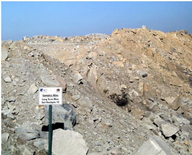
Figure #3. Soil and slightly acidic, brown, weathered sandstone from within 10 feet of the surface stockpiled, ready for distribution as the growth medium in West Virginia.
