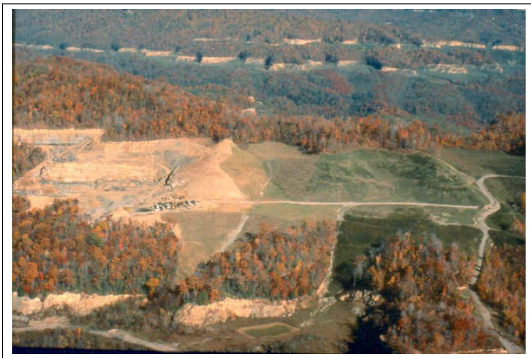
Figure 2. Appalachian coal mined landscapes of varying ages and mining methods in Wise County, Virginia. The active mine in the center of the photo is a conventional contour haul-back operation where the highwalls are backfilled to approximate original contour (AOC) with excess spoil disposed of in valley fills. The older pre-SMCRA mines in the immediate foreground and the background date to the 1960's and early 1970's and are clearly recognizable due to many linear km of exposed highwalls. Photo by Carl Zipper.
