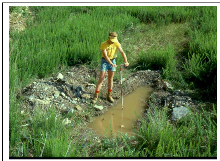
Figure 4. Wet mine soil in 1980. Subsoil was highly compacted and perching this saturated zone above approximately 20 m of unconsolidated spoil fill.
