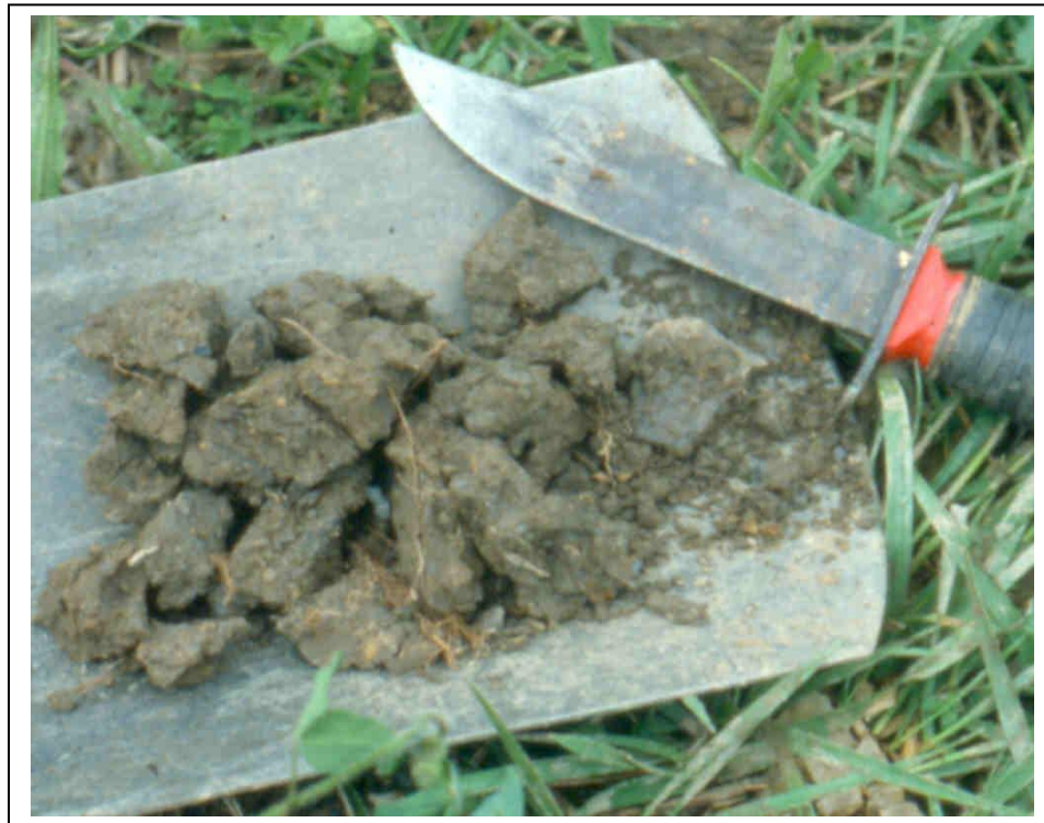
Figure 8. Moderate medium and coarse subangular and angular blocky aggregates broken out of the Bw horizon of a 12 year-old mine soil formed from a predominantly siltstone spoil.
