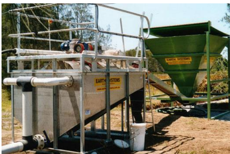
Figure 8. The HALT System. Low cost limestone gravel is fed to the system (foreground), from a storage hopper (background). Using a partly submerged modified rotating ball mill, the system grinds the limestone to produce an ultra fine grained slurry. The slurry is then dispensed into the receiving environment where reaction between the slurry and affected water body results in neutralization insitu .
