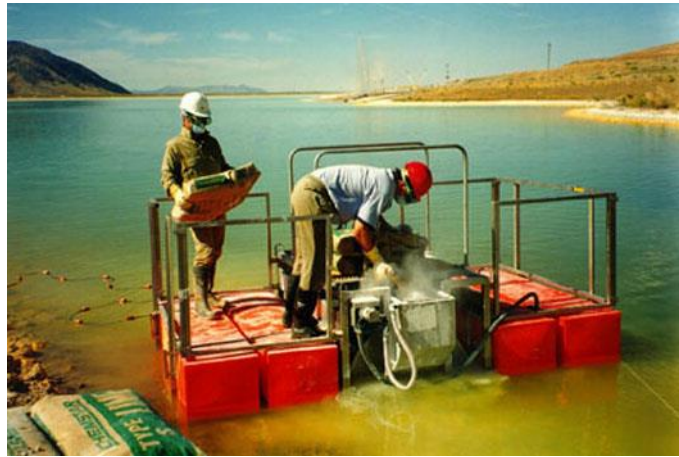
Figure 7. Treating a large tailings pond with a Neutra-Mill. The cloudy plume surrounding the floating mill is largely metal hydroxide precipitates from the reaction between the lime slurry being dispensed and the metalliferous ARD. For this treatment task the Neutra-Mill was loaded manually rather than using the automated reagent storage and delivery system.
