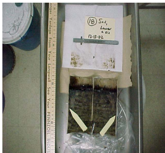
Figure 4. Oil permeation in lower (clay rich) soil after eight hours, with coal added to surface 30 minutes following oil addition. Note pattern of oil migration, detected with absorbent paper
