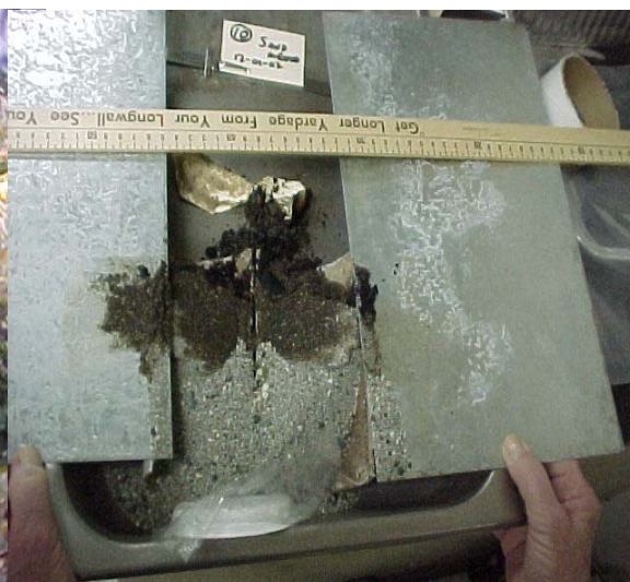
Figure 2. Sand sample, showing method of splitting for inspection. Note oil permeation pattern, and agglomerated coal layer at top of sample
