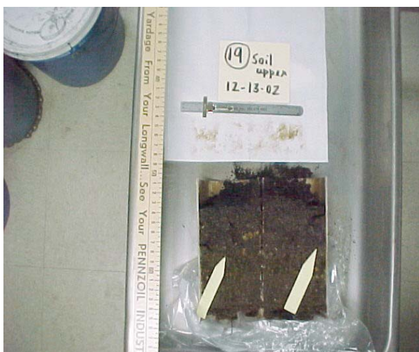
Figure 3. Oil permeation in upper (organic-rich) soil after 24 hours, with coal added to surface 30 minutes following oil addition. Note pattern of oil migration, detected with absorbent paper
