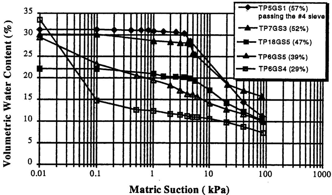
Figure 4. SWCC for soils in figure 3, Newman et al. (1997).
