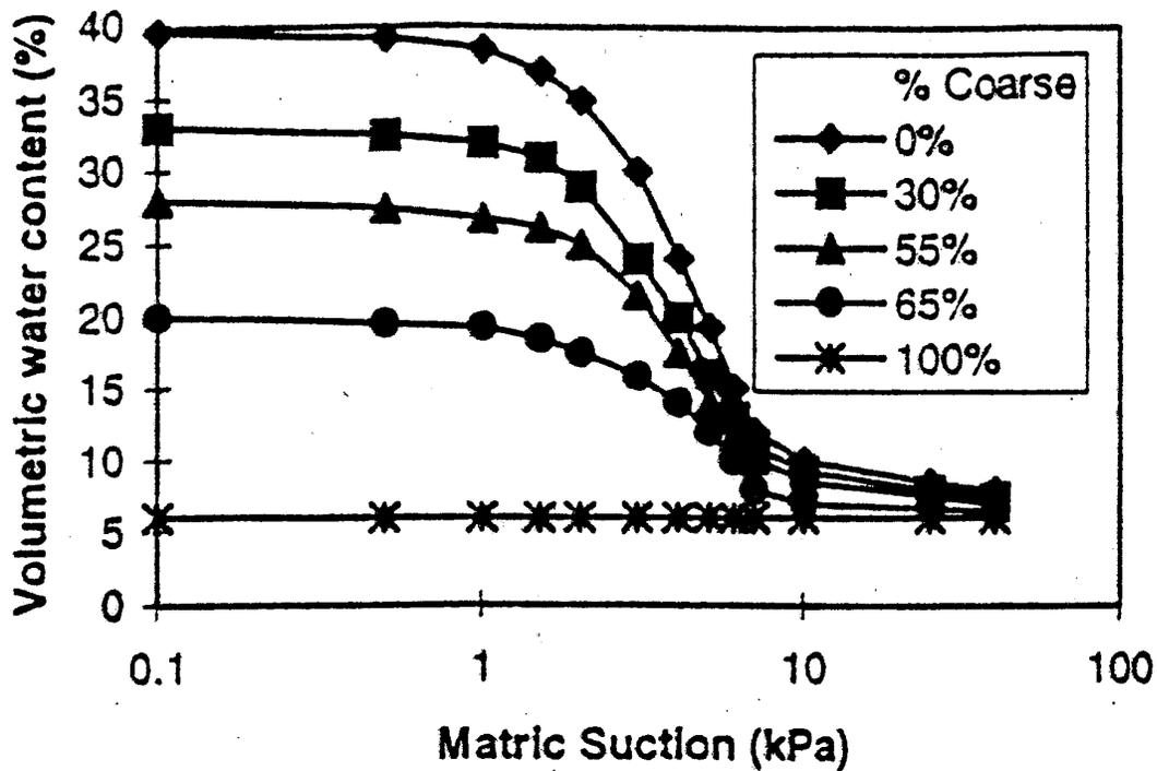
Figure 6. SWCC results for soils in Figure 5, Yazdani, et al.
