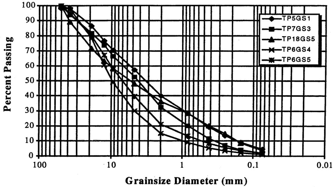
Figure 3. Grain-Size-Distribution curves for samples from Newman et al. (1997).
