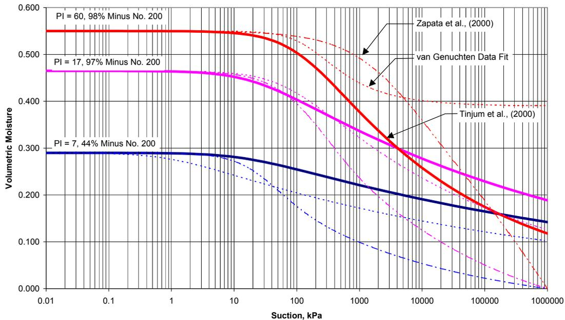
Figure 7. Effect of Plasticity on SWCC for three soils. Soil data from Miller et al., (2002) Standard Compaction Effort, Plus 2-percent Moisture. Calculations after Zapata et al., (2000) and Tinjum et al., (2000).
