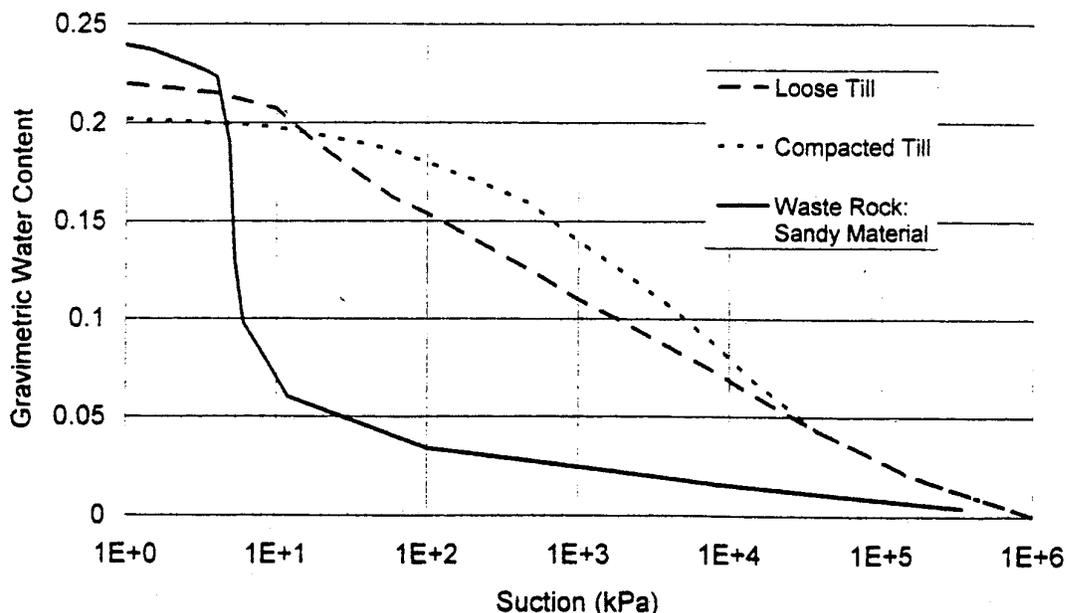
Figure 8. Typical effect of compaction in SWCC curves. From Wilson et al., (1995).
