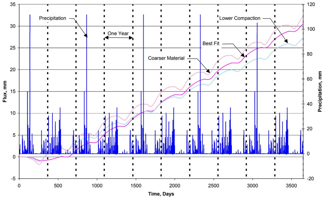
Figure 13. El Paso Sand cumulative flux and precipitation.
