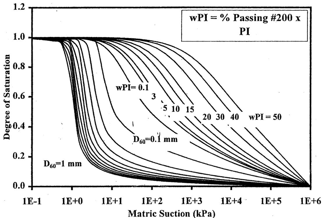
Figure 2. Predicted SWCC based on  $D_{60}$  and wPI, Zapata et al., (2000)
