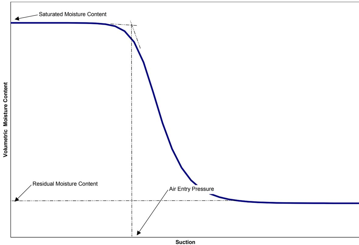
Figure 1. Typical Soil Water Characteristics Curve
