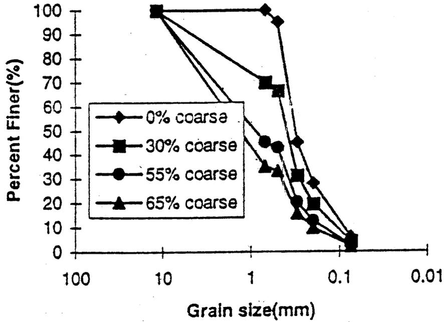
Figure 5. Grain-Size-Distribution of soils tested for SWCC by Yazdani, et al. Coarse is defined as particles retained on the No. 4 sieve.
