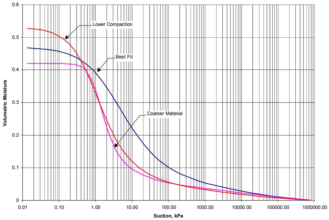
Figure 9. El Paso Sand SWCCs used in parametric study.
