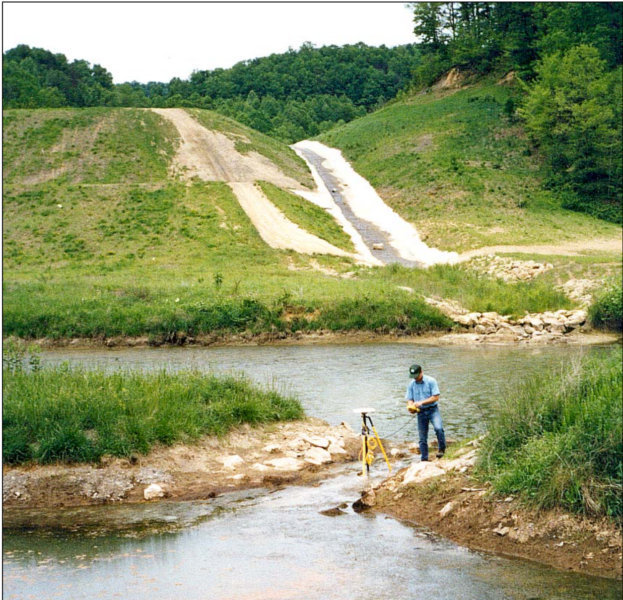
Figure 3: TIPS team member Kyle Bohnenstiehl surveys pond elevation in Tennessee with the GPS Total Station. A valley fill of removed mine overburden is in the background.
