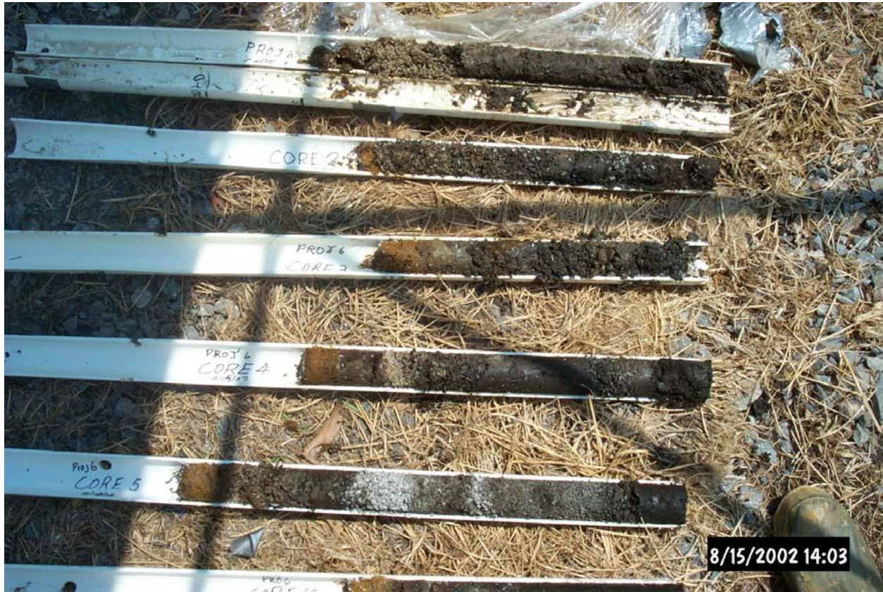
Figure 1: Photograph of sample cores after removal from the vertical flow pond.
