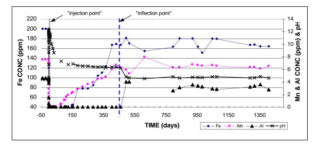
Figure 1. Concentrations of iron, aluminum, manganese, and pH verses time for the mine discharge for 4 years post injection.
