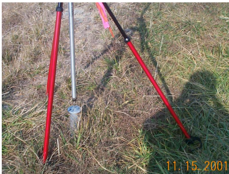
Figure 3. A survey monument buried in soil.
