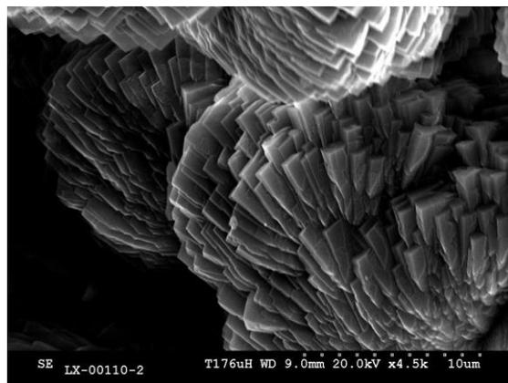
Figure 7. SEM image of calcite formed on the edge of the Big Gorilla mine pool (4500X).
