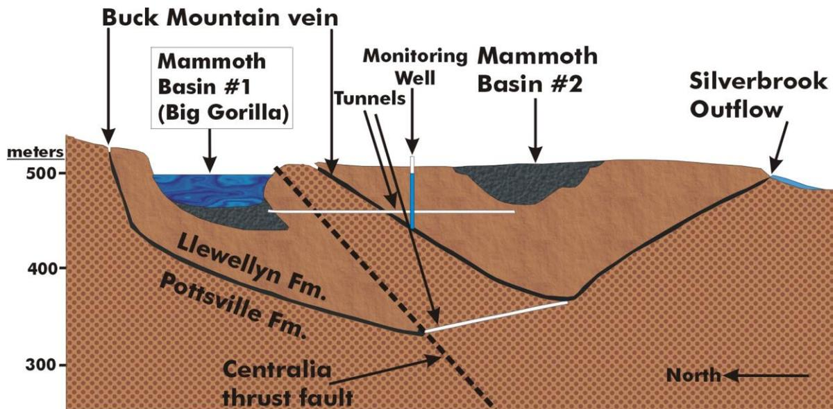
Figure 3. Cross-section of the Silverbrook Basin, constructed from a mine map by J.H. Winters, date unknown. The two Mammoth basins show the former location of the removed Mammoth seam.
