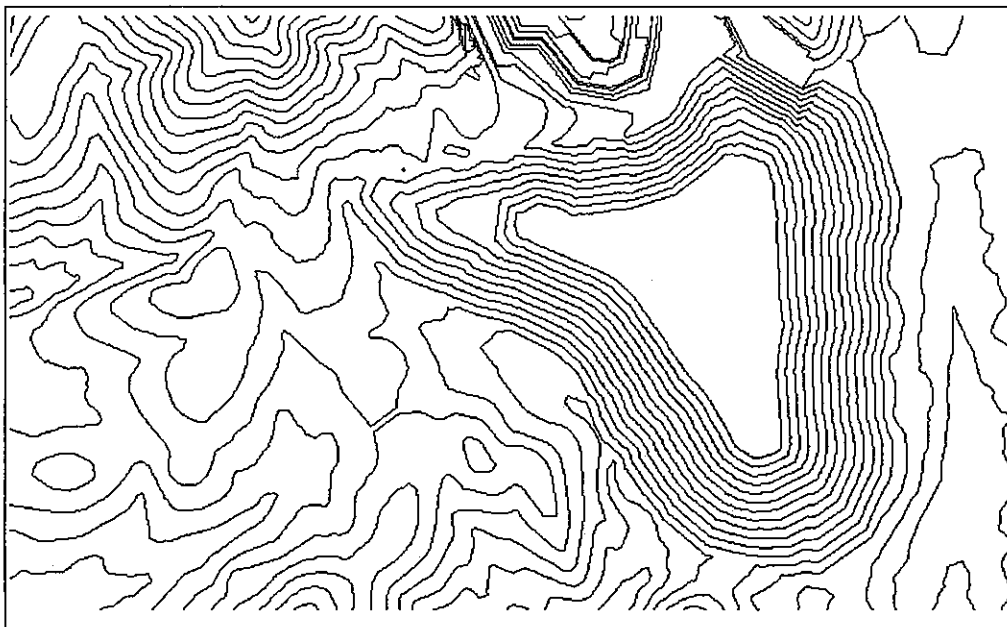
Figure 2. Raw topography data used to build a TIN
