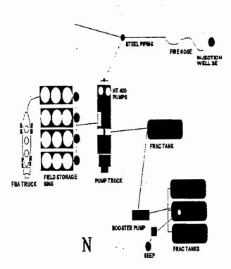
Figure 2. A depiction of the arrangement of the equipment used during the injection process.
