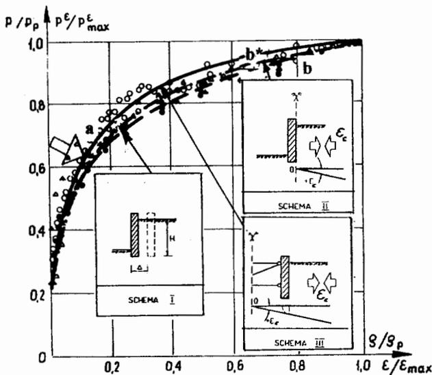
Figure 7. Engagement of the resultant soil pressure - soil thrust force on construction's supports for the non-dimensional coordinates. Diagrams : I- passive soil pressure (a), II- mine-induced compacting strain (b), III- two-sided soil thrust (b\*).
