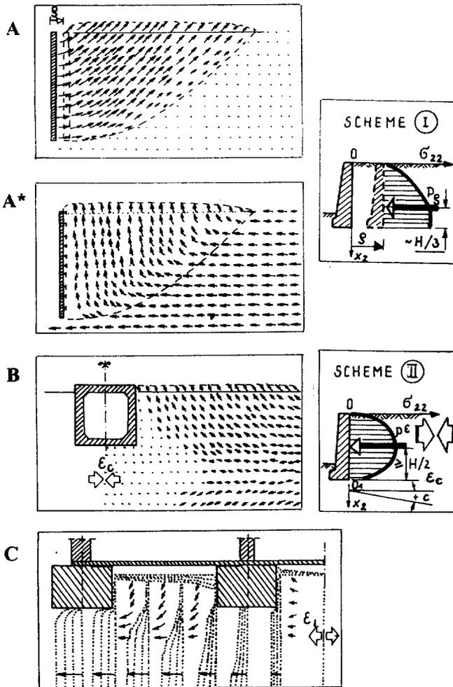
Figure 3. Vectorial displacement fields in the ground medium of Taylor-Schneebeilly type.
