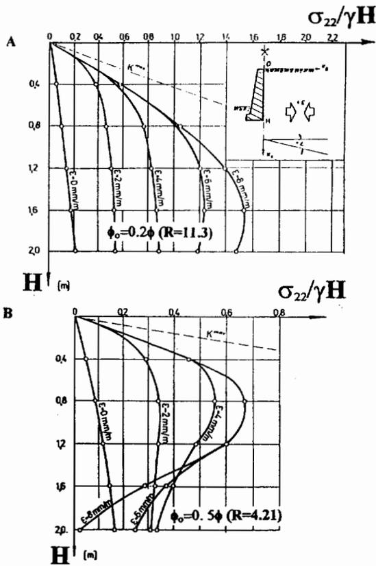
Figure 5. Theoretical increase of the one-sided thrust on the construction : A- smooth wall, B-rough wall
