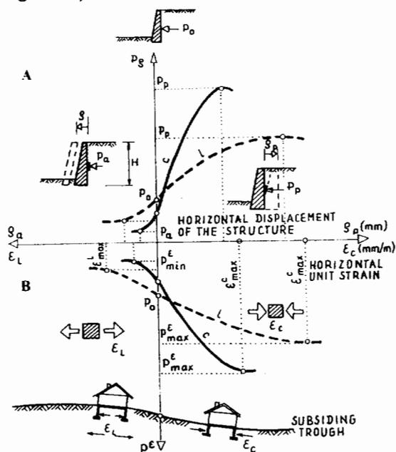
Figure 1. Influence of displacements or mine-induced strains  $\epsilon$  on the engagement of soil pressure  $P$  (soil thrust) for loose soil.
