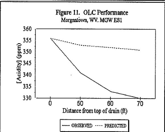
**Figure 11.** Observed and predicted acidity reductions of an open limestone channel at the Morgantown Airport east drain.
