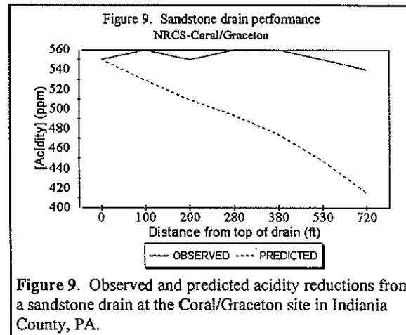
Figure 9. Observed and predicted acidity reductions from a sandstone drain at the Coral/Graceton site in Indiania County, PA.
