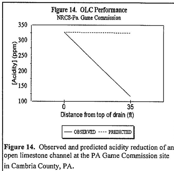
**Figure 14.** Observed and predicted acidity reduction of an open limestone channel at the PA Game Commission site in Cambria County, PA.
