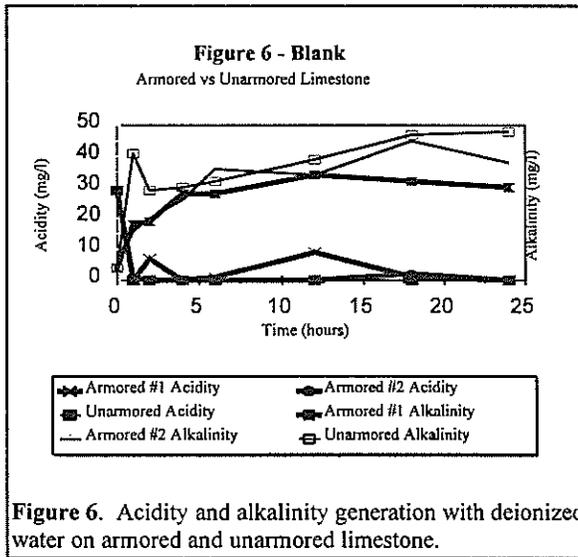
Figure 6. Acidity and alkalinity generation with deionized water on armored and unarmored limestone.
