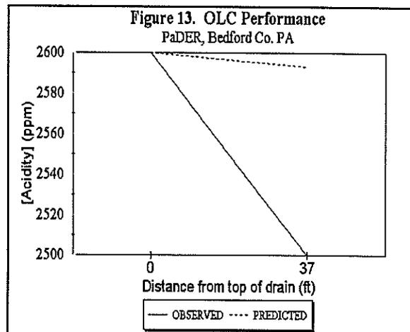
**Figure 13.** Observed and predicted acidity reductions of an open limestone channel at the Pa DER site in Bedford County, PA.
