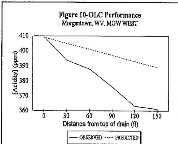
**Figure 10.** Observed and predicted acidity reductions of an open limestone channel at the Morgantown Airport west drain.
