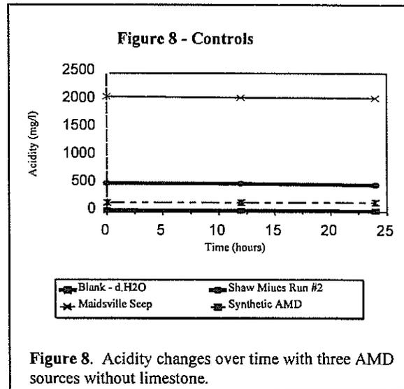
Figure 8. Acidity changes over time with three AMD sources without limestone.
