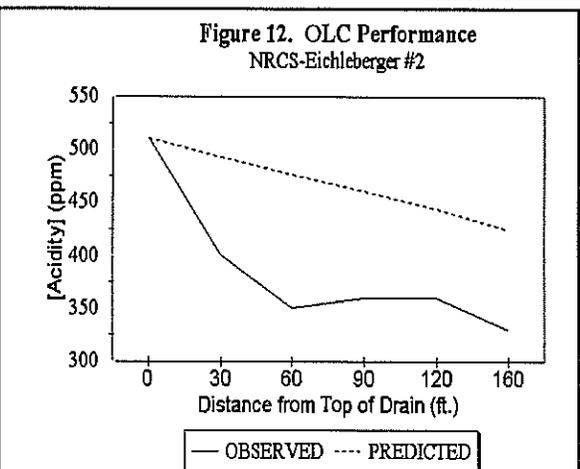
**Figure 12.** Observed and predicted acidity reductions of an open limestone channel at the NRCS Eichleberger #2 site in Bedford County, PA.
