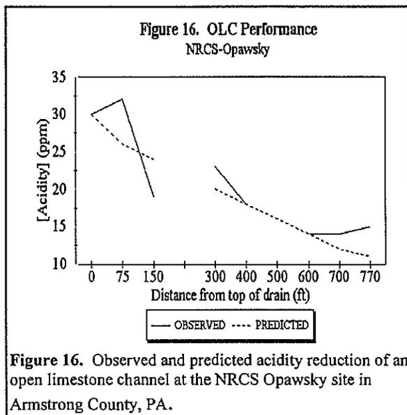
The NRCS Opawsky site's performance was slightly worse than predicted (0.33% acidity removal per ft compared to a predicted removal of 0.42% per ft) but still removed 50% of the acidity (Figure 16).
