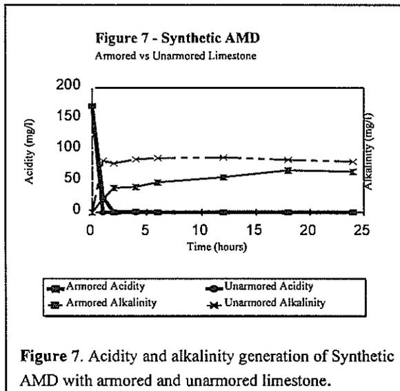
Figure 7. Acidity and alkalinity generation of Synthetic AMD with armored and unarmored limestone.
