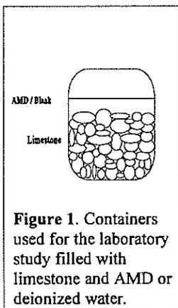
**Figure 1.** Containers used for the laboratory study filled with limestone and AMD or deionized water.
