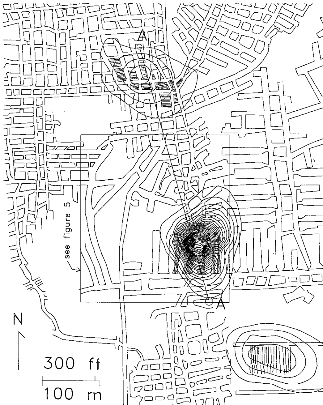
Figure 3.-Estimated subsidence contours with hypothetical associated pillars shaded, minimum contour is 0.05 m, contour interval is 0.025 m; see figure 4 for location.
