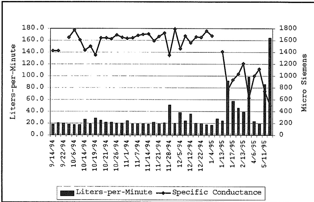
Figure 2. Discharge and Specific Conductance measurements for monitoring point No. 3, Case Study 1.
