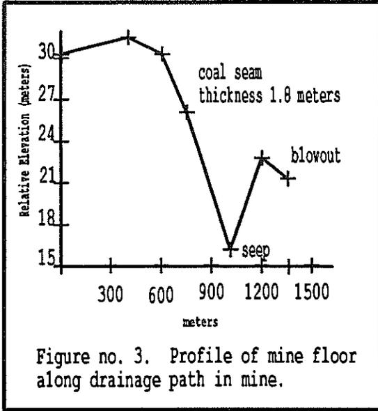
Figure no. 3. Profile of mine floor along drainage path in mine.
