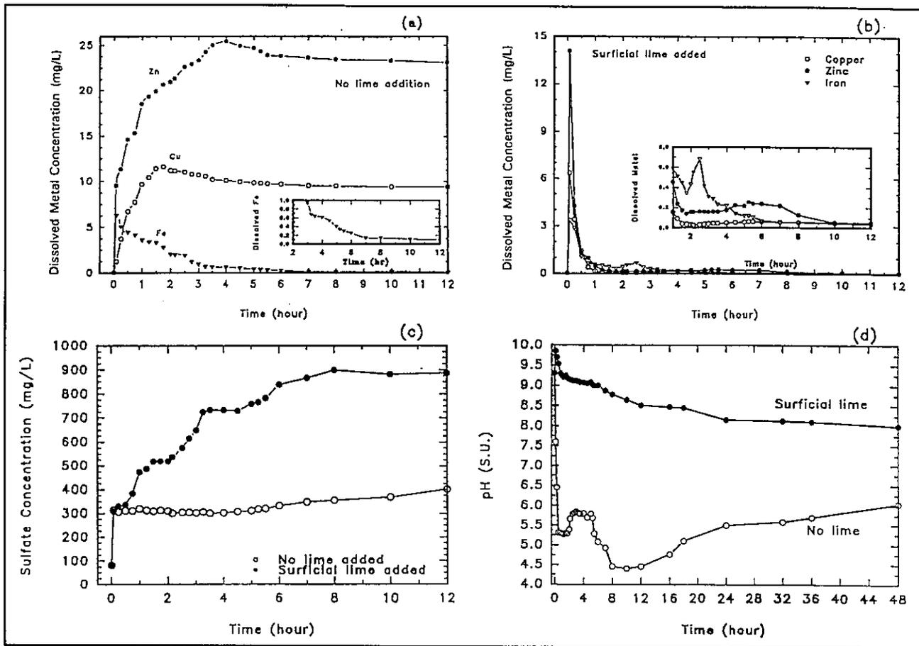
Figure 2. a) Metal release with time for flooded tailings, no lime addition. b) Metal release with time from flooded tailings, surficial lime addition. c) Effect of surficial lime additions on sulfate release. d) Solution pH with time for lime and no lime treatments.
