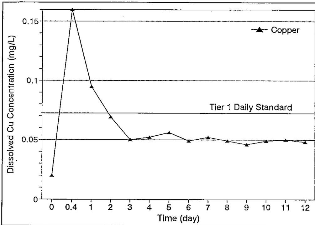
Figure 3. Copper concentration with time for exposed tailings receiving surficial lime slurry treatment.
