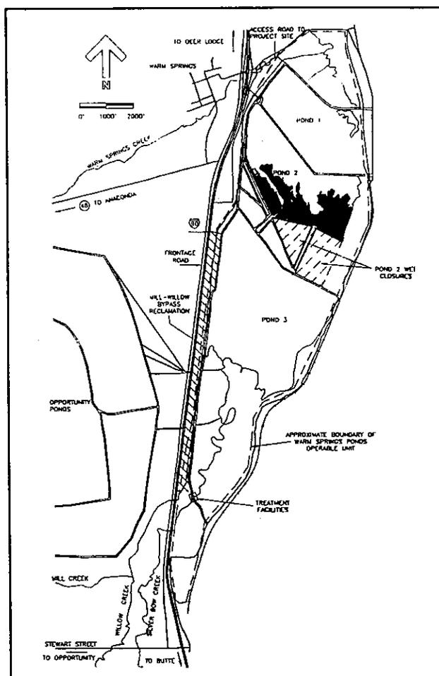
Figure 1. Site location and map for Pond 2 wet-closure study, Warm Springs Ponds. Shaded area represents exposed tailings that were wet closed.
