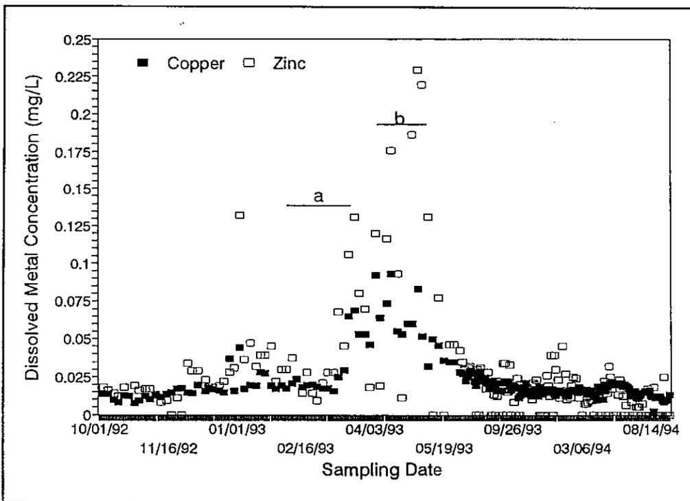
Figure 4. Dissolved metal concentration in Pond 2 discharge. a) Period of Pond 2 raise. b) Period of Pond 2 bypass, no discharge Pond 2.
