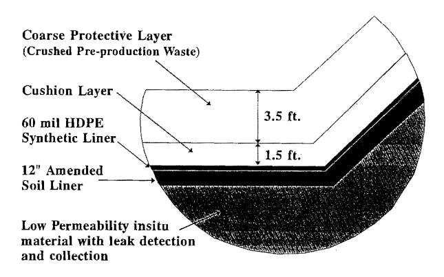
Figure 1. Schematic diagram of the composite liner.
