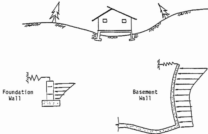
Figure 3. Schematic of plane strain idealization of compression zone (Drumm et al. 1988).
