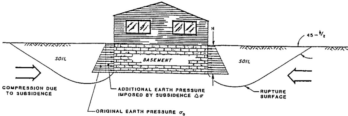
Figure 1. Earth pressure on subgrade walls of building located in compressive subsidence zone (Speck and Bruhn 1990).
