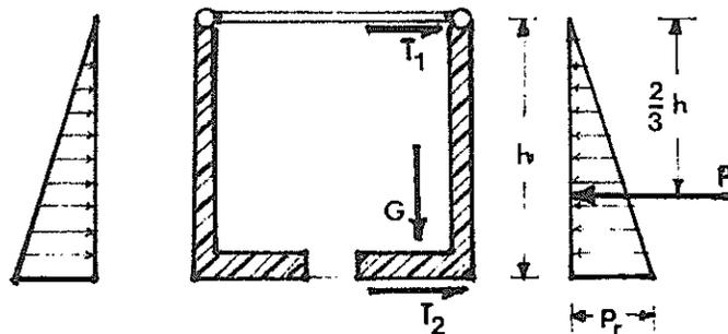
Figure 7. Schematic system of tunnel walls.
