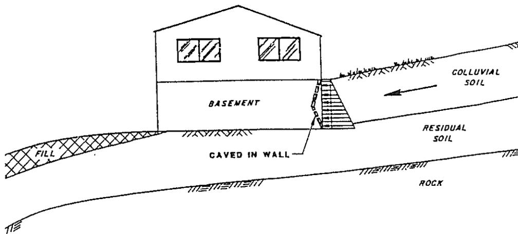
Figure 2. Earth pressure on uphill subgrade wall of building intensified by subsidence-induced hillslope instability (Speck and Bruhn 1990).
