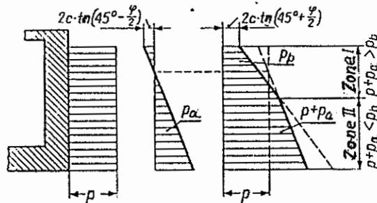
Figure 5. Pressure on wall in zone of compressive strain.
