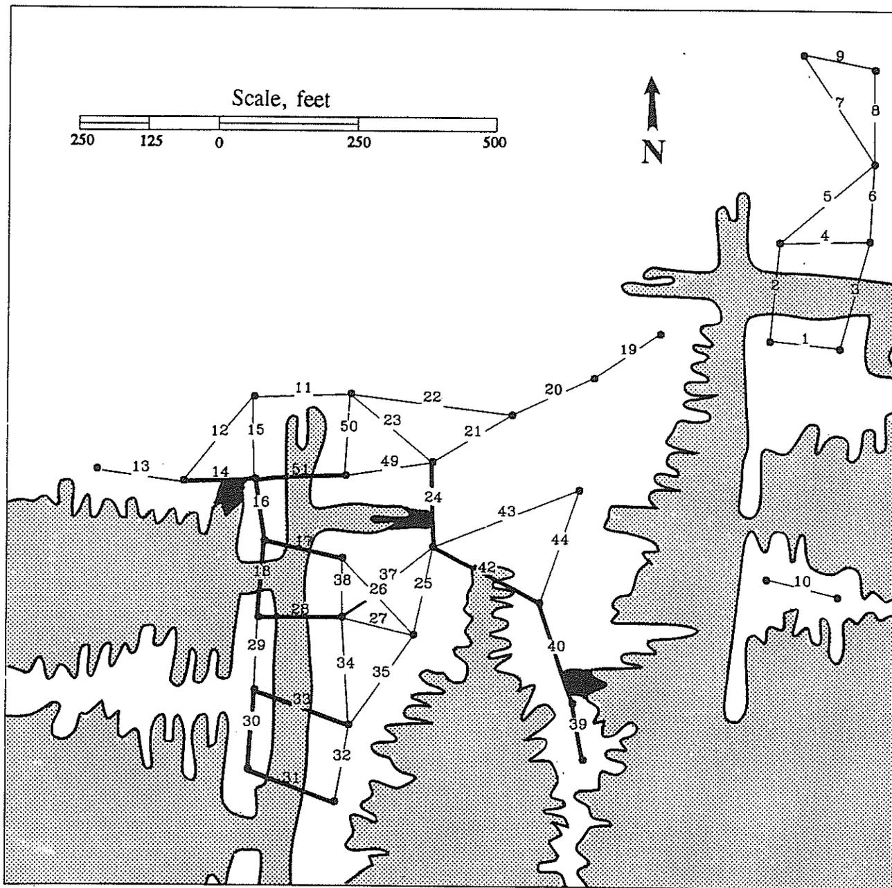
Figure 4. Map showing mine outline of the Carlisle Coal Mining Co. Mine No. 1, interpreted from the original 1928 map, and the RIM survey. Solid lines show ray paths identified by number. Shaded areas represent believed worked areas. Small circles are boreholes drilled through the coal seam. Multiple-frequency analysis ray paths are bold lines. Solid areas are mining identified by RIM and not on original map.
