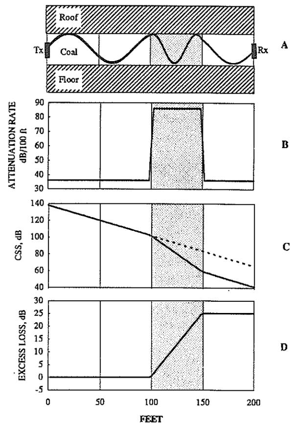
Figure 1. Diagram of the RIM transmission and analysis curves in a coal seam with water filled void (shaded area). A) EM wave in a coal seam, width of line indicates decreasing signal amplitude. Antennae are denoted by  $T_x$  and  $R_x$ . B) Attenuation rates in coal seam and mine void. C) CSS, corrected signal strength of the EM wave as it passes through seam with workings present (solid line) and in absence of workings (dashed line). D) Excess loss of the EM wave in the seam.
