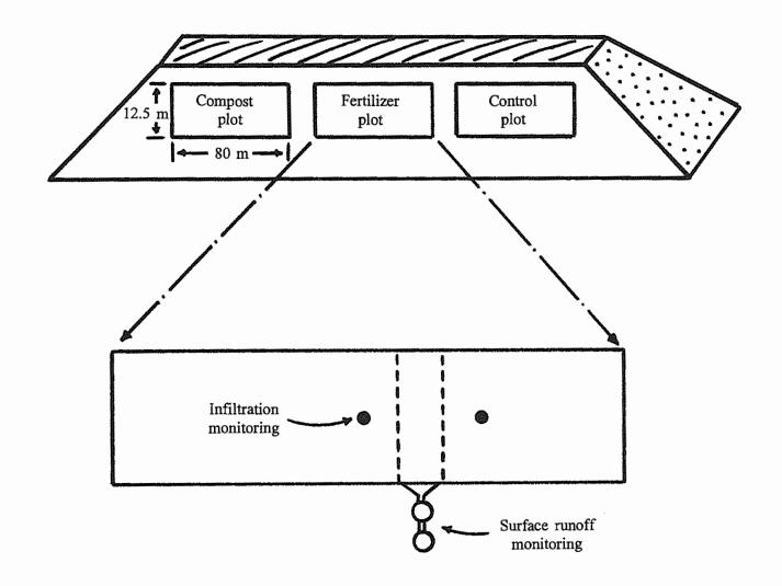
Figure 1. Test plot design and sample locations.
