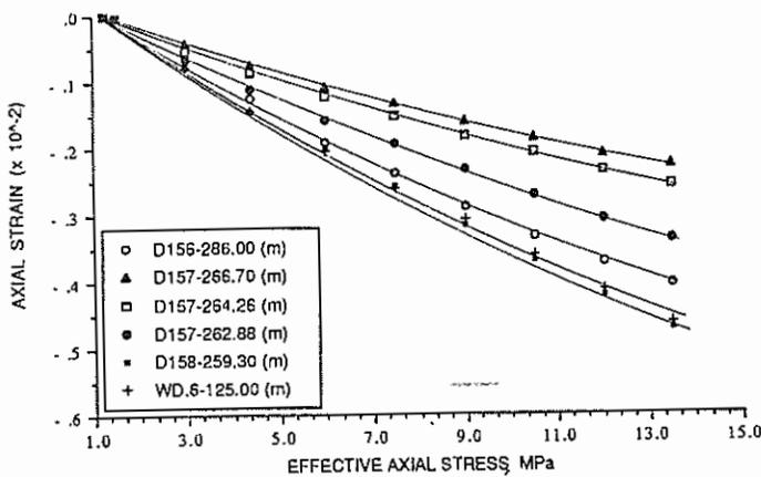
Figure 6. Relationship between axial strain and effective axial stress for first loading.
