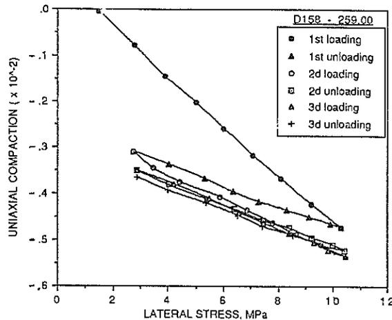
Figure 5. Typical lateral stress-strain compaction relationship with three loading cycles.
