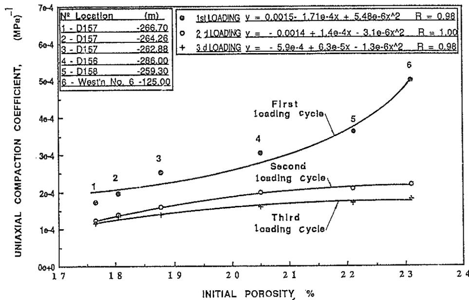
Figure 8. Relationship between uniaxial compaction coefficient and initial porosity for first, second and third loading.
