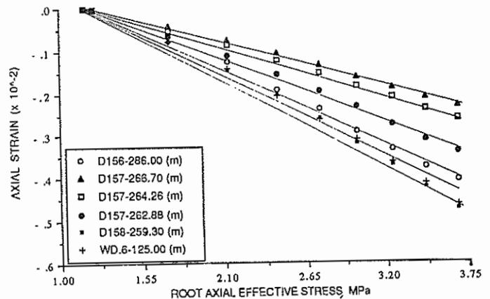
Figure 7. Relationship between axial strain and root of effective axial stress for first loading.
