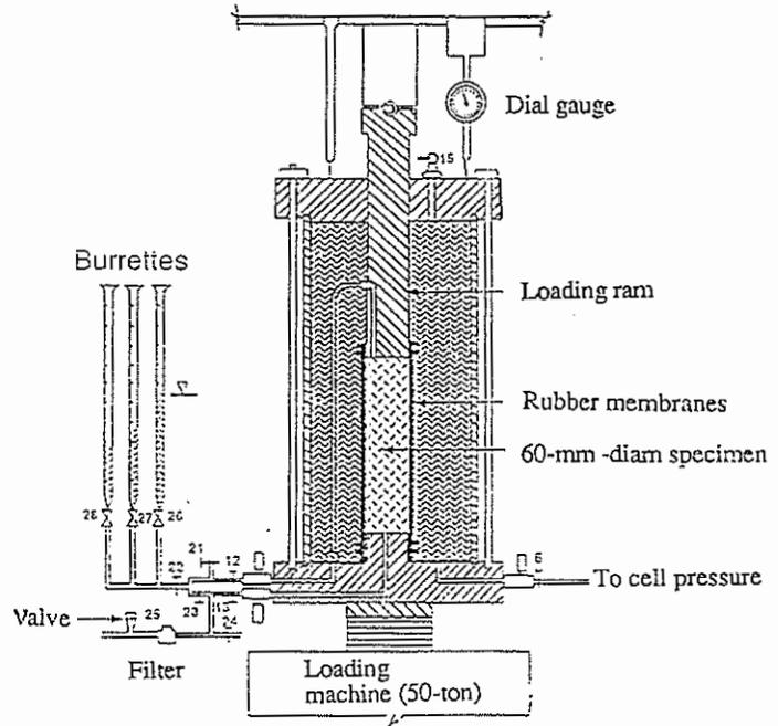
Figure 3. Arrangement of apparatus for compaction test.
