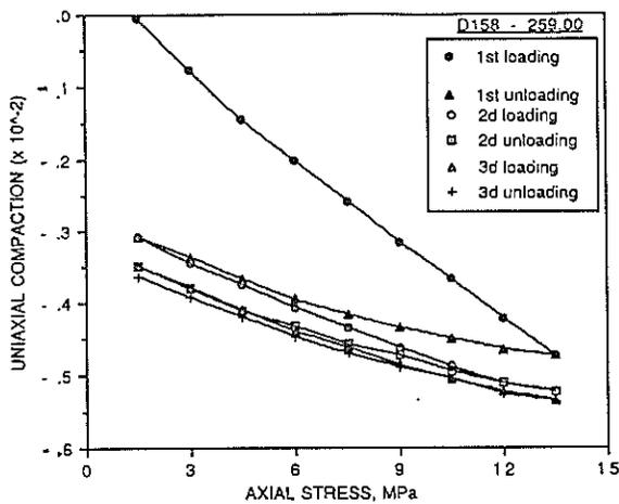
Figure 4. Typical axial stress-strain compaction relationship with three loading cycles.
