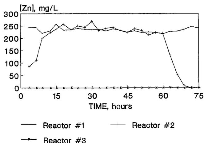
Figure 4. Chemical stage dissolved zinc levels during 75 hour continuous AMD treatment.
