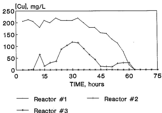
Figure 3. Chemical stage dissolved copper levels during 75 hour continuous AMD treatment.
