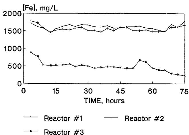
Figure 5. Chemical stage dissolved iron levels during 75 hour continuous AMD treatment.
