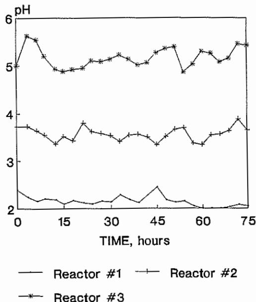
Figure 2. Chemical stage pH values during 75 hour continuous AMD treatment.
