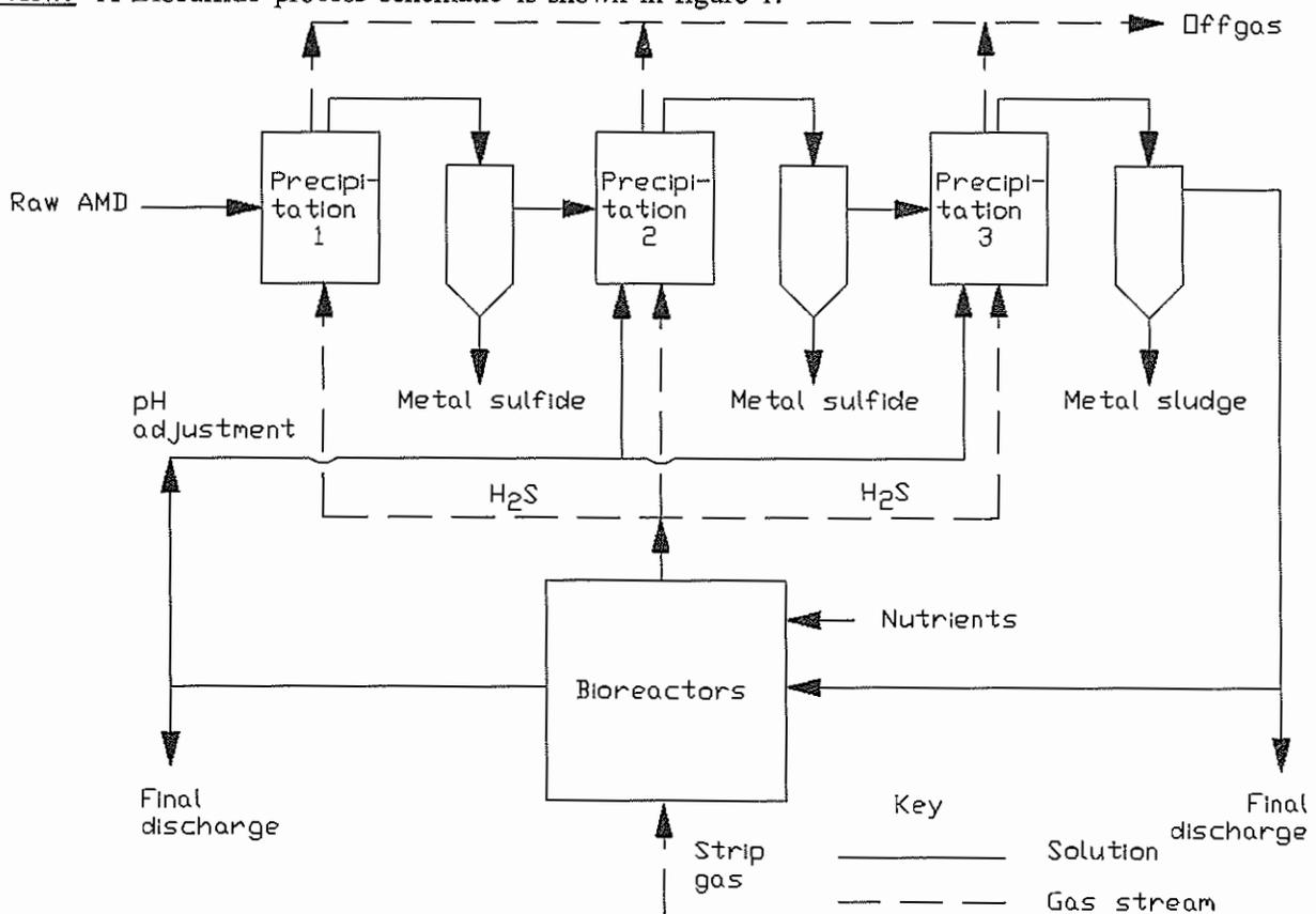
Figure 1. Biosulfide process schematic.
