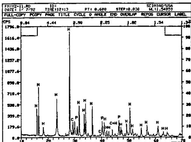
Figure 2. X-ray diffractogram of scrubber sludge. (C = Calcium carbonate, H= Calcium sulfate hydrate, P = Pyrite)
