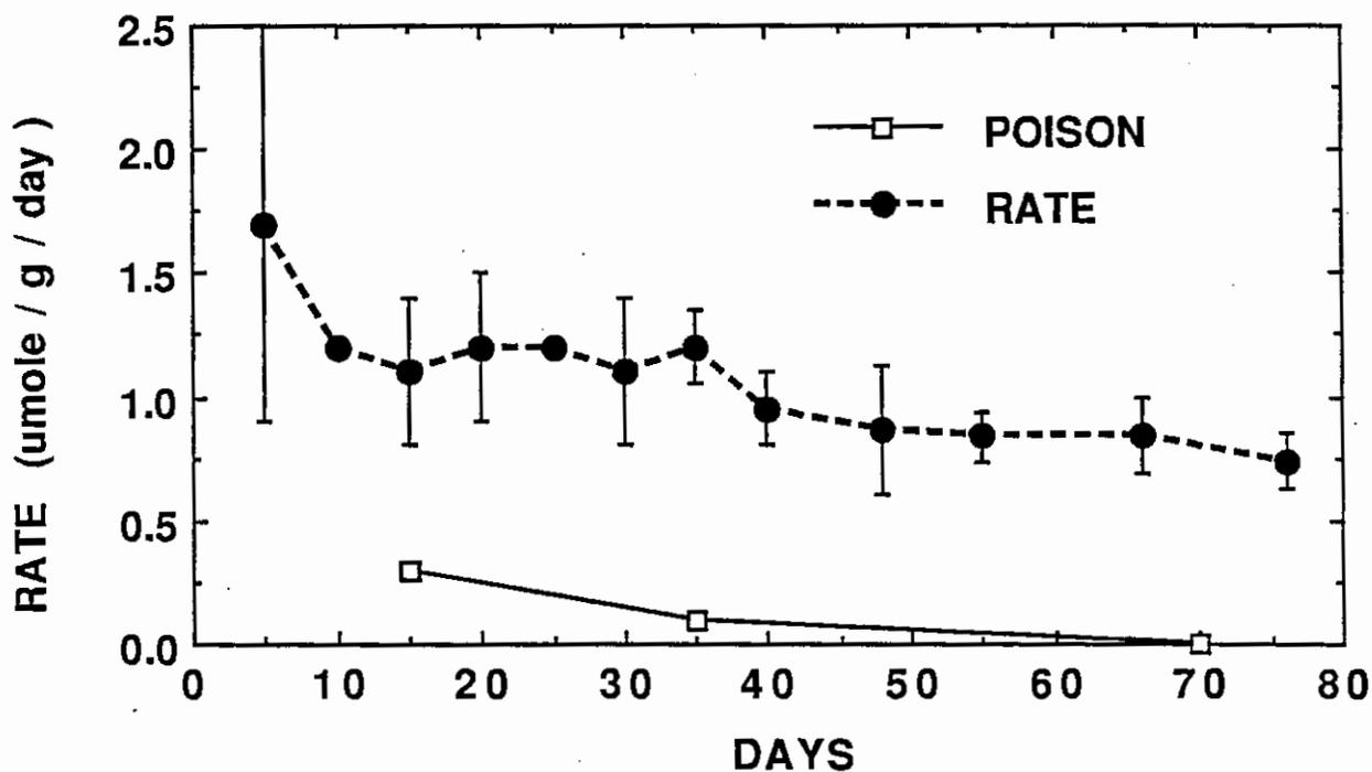
FIGURE 1. Rate of Sulfide Production in Serum Bottles and Poisoned Controls. Error bars represent one standard deviation. Data points without error bars are the average of two samples.
